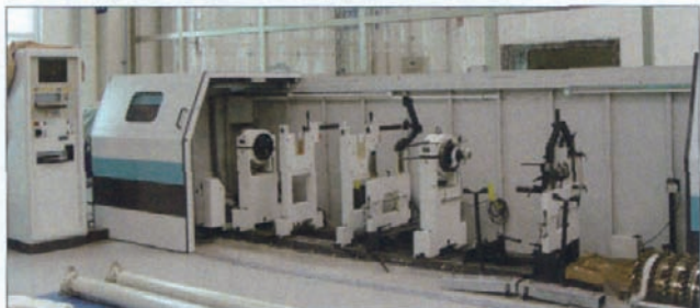
图3 德国HK4卧式平衡机 Fig.3 HK4 horizontal balancing machine made in Germany
